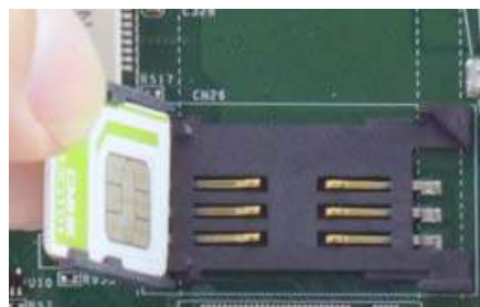
Insert Mini-SIM card with pins facing up
