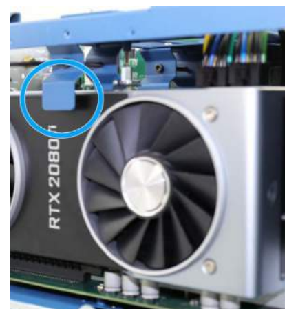
Make sure bracket DOES NOT OBSTRUCT graphics card's fan
