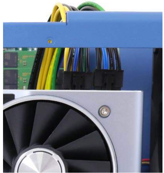
6 or 8-pin power connector on graphics card
