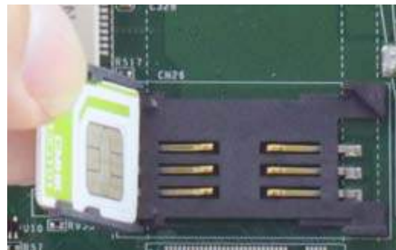
Insert Mini-SIM card with pins facing up
