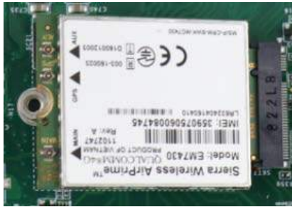
Insert on 45 degree angle
